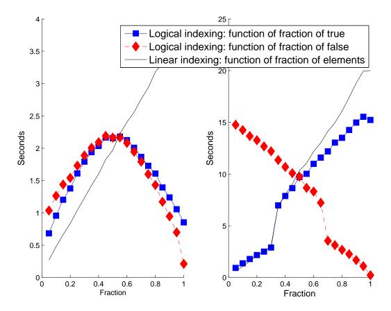
Figure 6: Analysis of the optimal proportion of using linear indexing vs. logical indexing as a function of proportion of true or false. The left panel is for v = 2, while the right panel is for v = 10.
