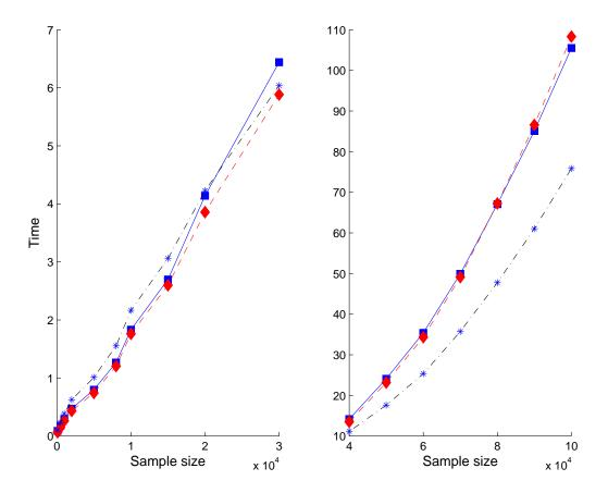
Figure 7: Analysis of computation time of three ways of multiplying matrices. The line with marker \* is associated with implementation based on Equation 13, while lines with square and diamond markers use, respectively, Equations 14 and 12.
